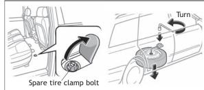
Removing the spare tire (all-wheel drive models)
